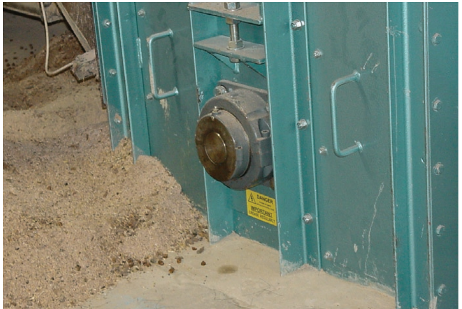
A Cooper square flange bearing arrangement in the dusty environment on a grain elevator
