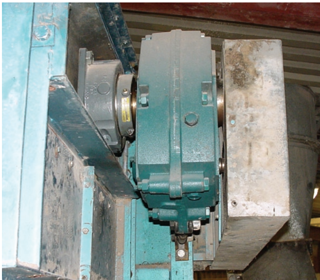
A Cooper square flange in a trapped drive position
